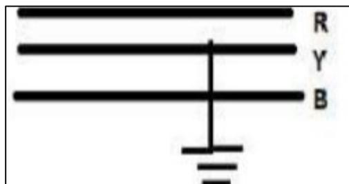
Fig. 3: Line to ground fault
