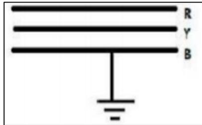
Fig. 1: Single line-to-ground fault
