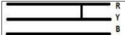
Fig. 2: Line to Line Fault
