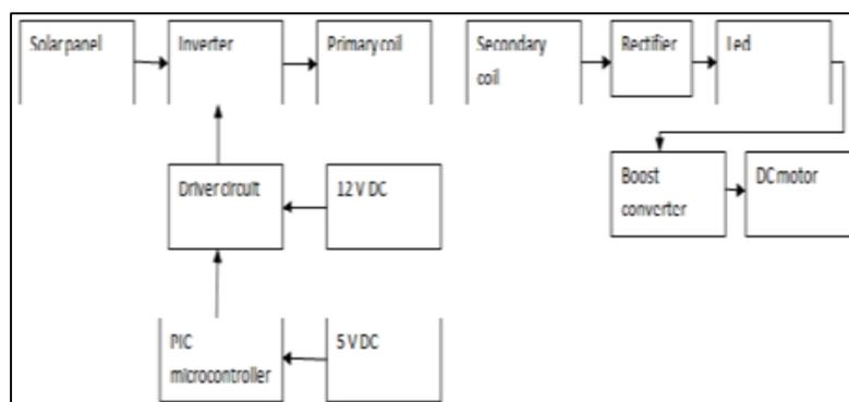
Fig. 1: Block of Wireless Power Transmission
