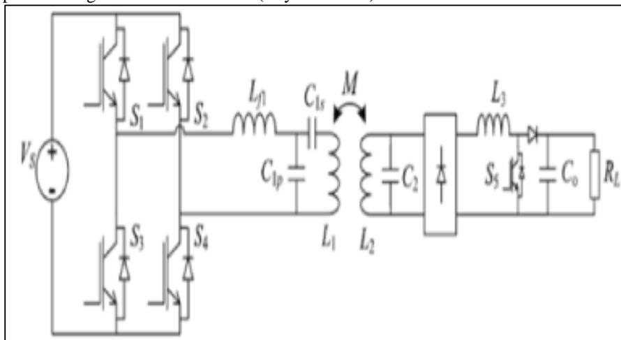
Fig. 4: Circuit of Wireless Power Transfer
