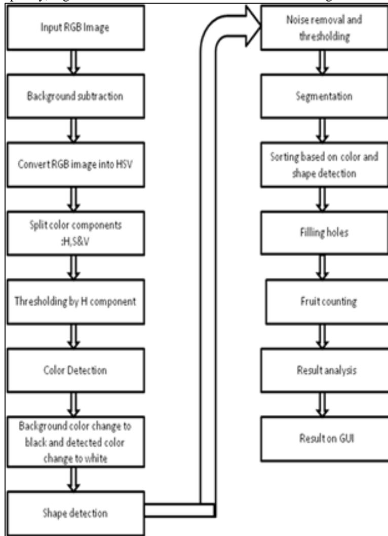
Fig. 4: Block diagram of the proposed system
