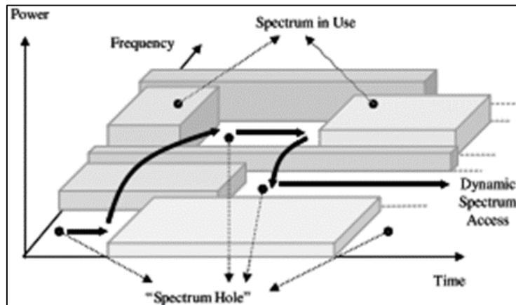
Fig. 2: Spectrum hole concept [7]
