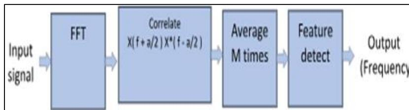
Fig. 4: Block diagram of Cyclostationary feature detection
