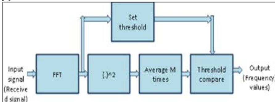
Fig. 3: Block diagram of energy detection
