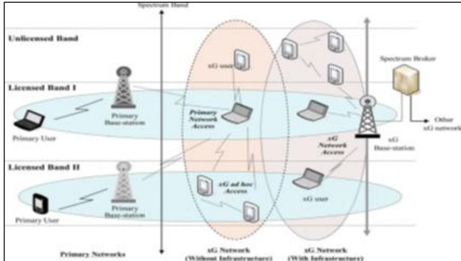
Fig. 1: cognitive radio architecture [10]
