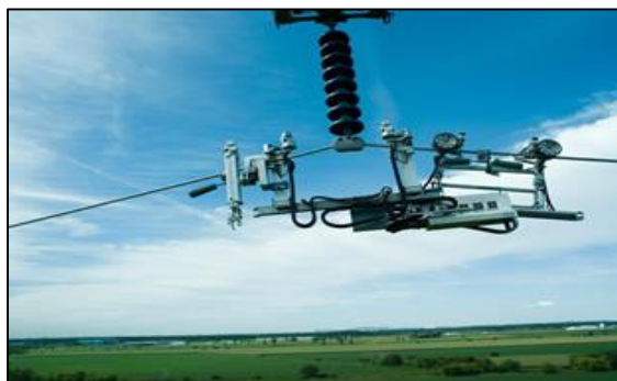
Fig. 7: Line inspection robot
