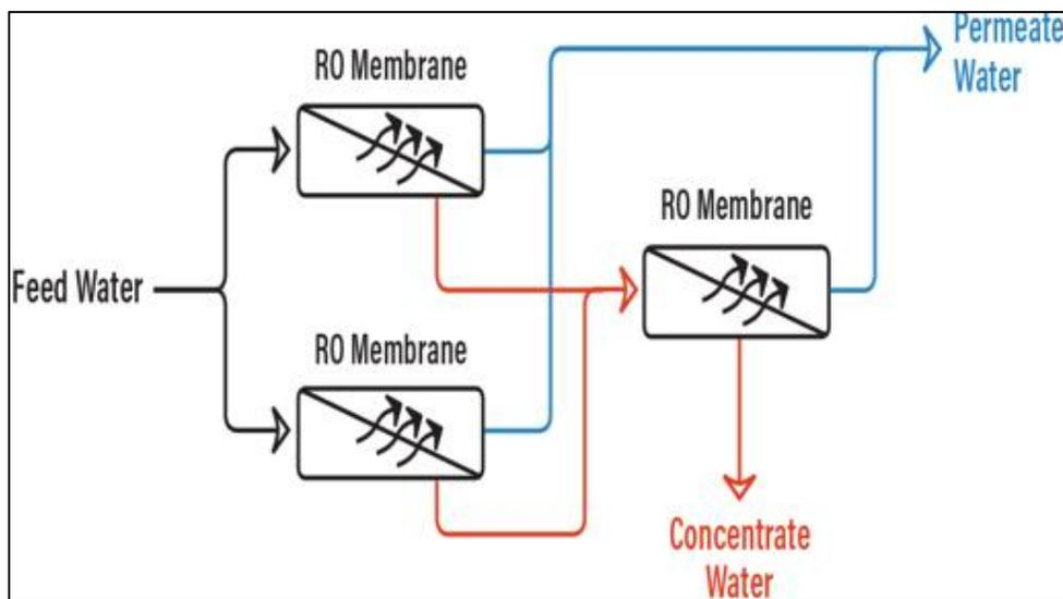
Fig. 8: 2<sup>nd</sup> Stage of RO System
