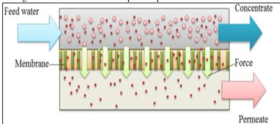
Fig. 1: Mechanism of membrane to concentrate and separate feed water
