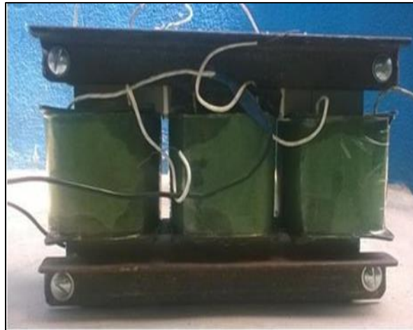
Fig. 8: Prototype model of three phase 1KVA 415/230V \gamma/\Delta distribution transformer with High grade M19 silicon steel
