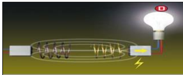
Fig. 6: receiving coil, lighting the bulb
