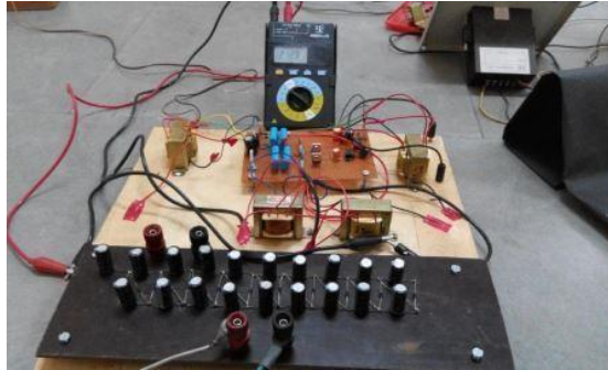
Fig. 9: Cockroft Walton hardware Circuit
