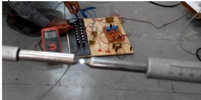
Fig. 10: Testing of Rod Gap Assembly by using Cockroft Walton Output
