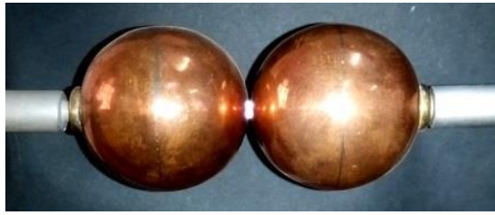
Fig. 11: Testing of Spheare Gap by using Cockroft Walton Output
