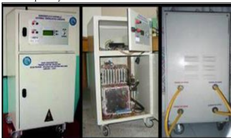
Fig. 2: microcontroller controlled geothermal thermoelectric generator
