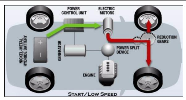
1) At start-off/low-speeds, Hybrid Synergy Drive runs the car on the electric motors only, since the gas/petrol engine does not perform efficiently. A gas/petrol engine cannot produce high torque in the low r.p.m. range, whereas electric motors can - delivering a very responsive and smooth start.
