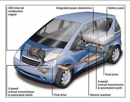
You can combine the two power sources found in a hybrid car in different ways. One way, known as a parallel hybrid, has a fuel tank that supplies gasoline to the engine and a set of batteries that supplies power to the electric motor. Both the engine and the electric motor can turn the transmission at the same time, and the transmission then turns the wheels.
