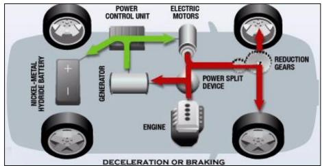
3) Under deceleration or braking, Hybrid Synergy Drive uses the car's kinetic energy to let the wheels turn the electric motors and recover regenerative energy to recharge the battery. Energy that is normally lost as friction heat under deceleration is converted into electrical energy, which is recovered in the battery to be reused later.
