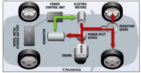
2) However, the gas/petrol engine is quite energy efficient for cruising. Power produced by the gas/petrol engine is used to drive the wheels and also the generator to provide power to the electric motors or to charge the battery. By making use of the engine/motor dual powertrain, the energy produced by the gas/petrol engine is transferred to the road surface with minimal loss.
