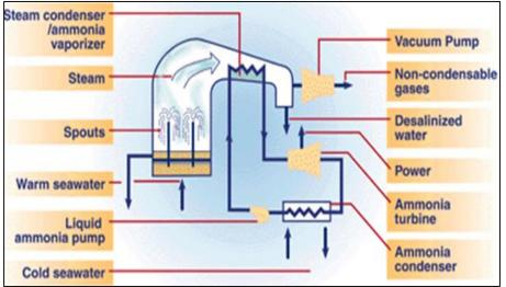
The steam vaporizes the ammonia working fluid of a closed-cycle loop on the other side of an ammonia vaporizer. The vaporized fluid then drives a turbine to produce electricity. The steam condenses within the heat exchanger and provides desalinated water. (sea heat pipe)
