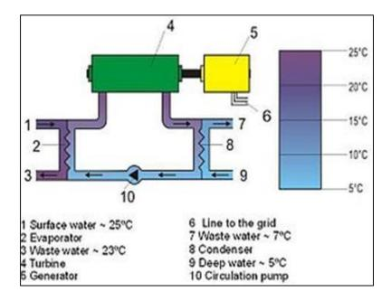
Closed-cycle systems use fluid with a low boiling point, such as ammonia, to power a turbine to generate electricity. Warm surface seawater is pumped through a heat exchanger to vaporize the fluid. The expanding vapor turns the turbo-generator. Cold water, pumped through a second heat exchanger, condenses the vapor into a liquid, which is then recycled through the system.
