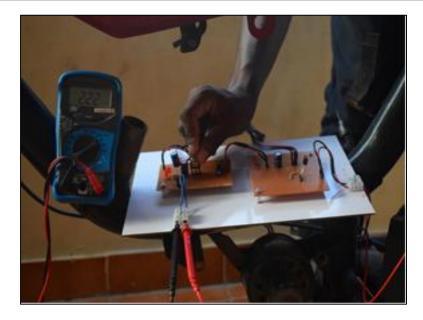
The maximum output voltage 2.22 volt, and the reading is been measured by the multimeter
