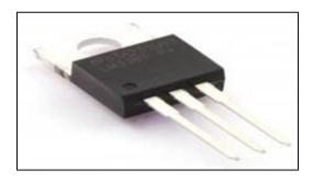
The LM138 series of adjustable 3-terminal positive voltage regulators is capable of supplying in excess of 5A over a 1.2V to 32V output range. They are exceptionally easy to use and require only 2 resistors to set the output voltage. Careful circuit design has resulted in outstanding load and line regulation comparable to many commercial power supplies. The LM138 family is supplied in a standard 3-lead transistor package.
