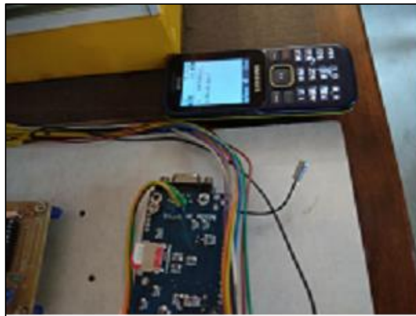
Fig. 6: critical message alert from GSM.
