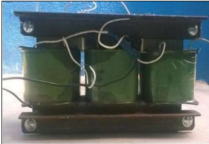
Fig. 8: Prototype model of three phase 1KVA 415/230V \gamma/\Delta distribution transformer with High grade M19 silicon steel
