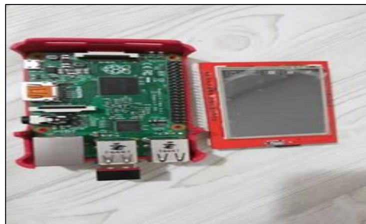
Fig. 5: Connecting back removed LCD to Raspberry PI
