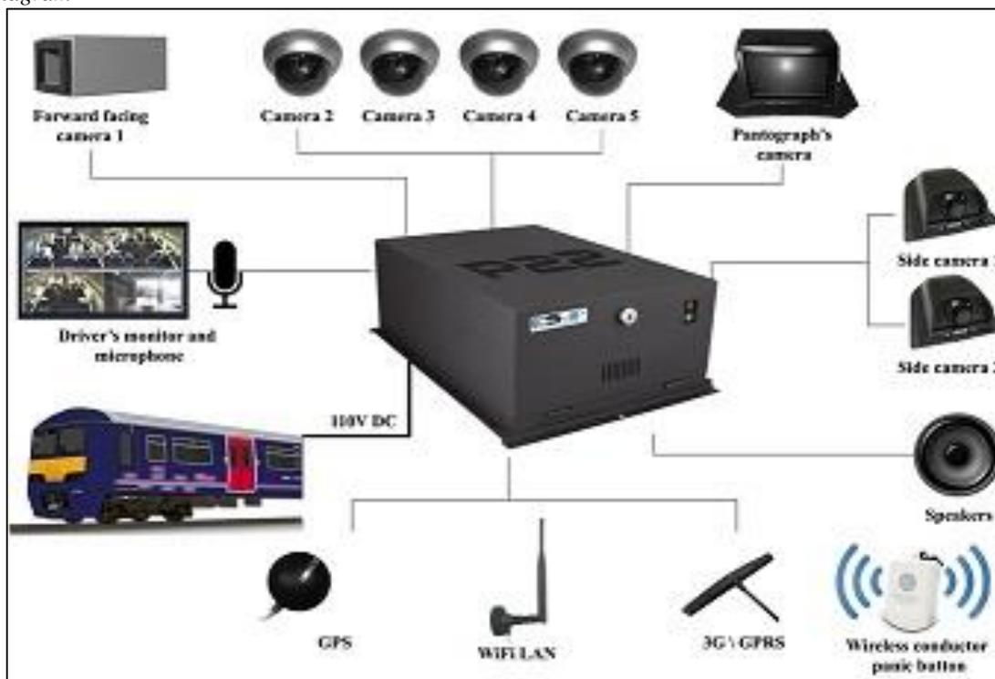
Fig. 2: Block Diagram of the Surveillance System
