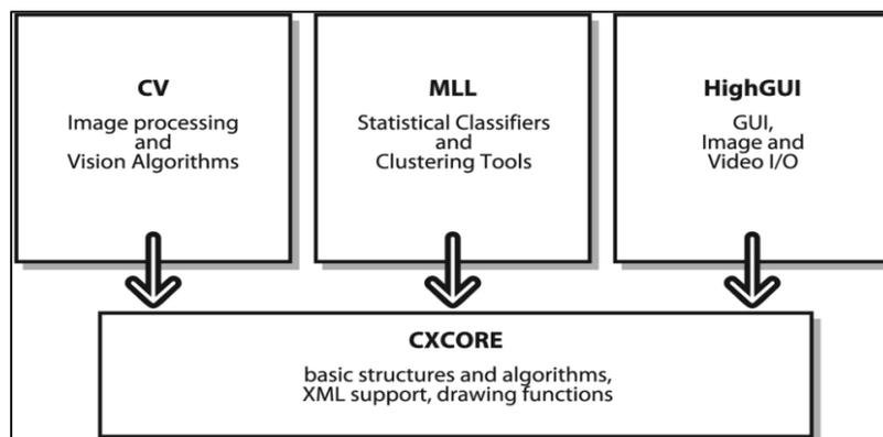
Fig. 1: Basic Structure of OpenCV
