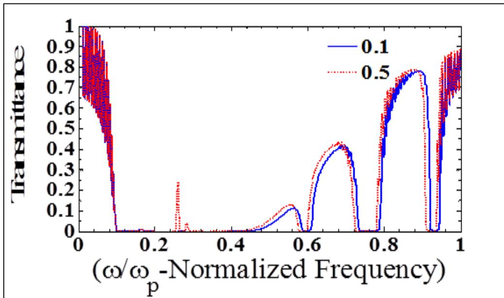
Fig. 3: Transmission spectra of PBG for  $\chi_p^{(3)} E_0^2 = 0.1$  and  $\chi_p^{(3)} E_0^2 = 0.5$  when  $f=0.4$  and  $r= 5$  nm
