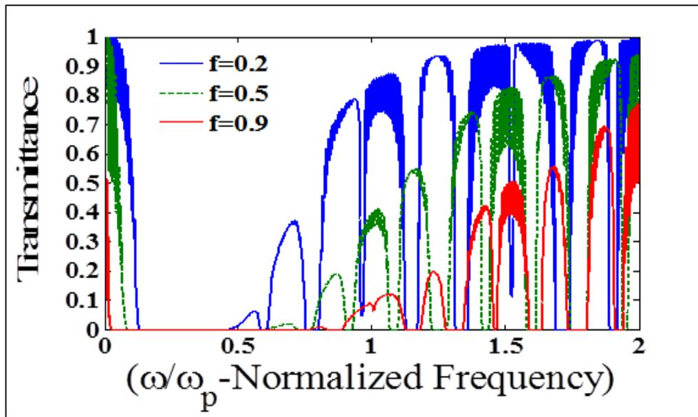
Fig. 1: Transmission spectra of PBG for filling factor  $f=0.2$ ,  $f=0.5$  and  $f=0.9$  when  $r=2$  nm,  $\chi_p^{(3)} E_0^2 = 0.1$
