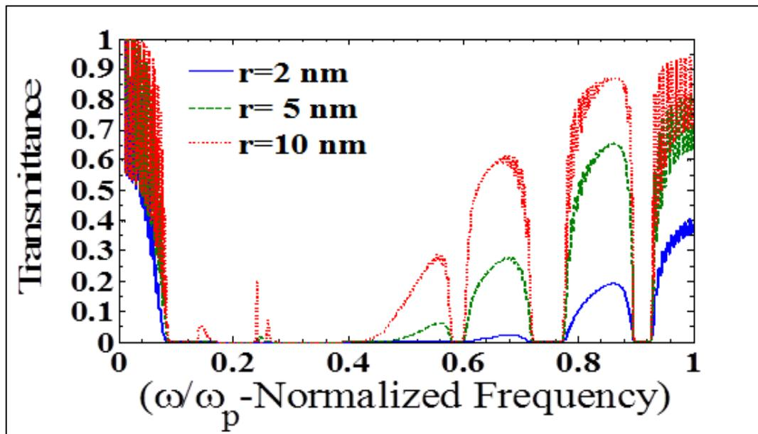
Fig. 2: Transmission spectra of PBG for radii 2 nm, 5 nm and 10 nm when  $f=0.5$ ,  $\chi_p^{(3)} E_0^2 = 0.3$
