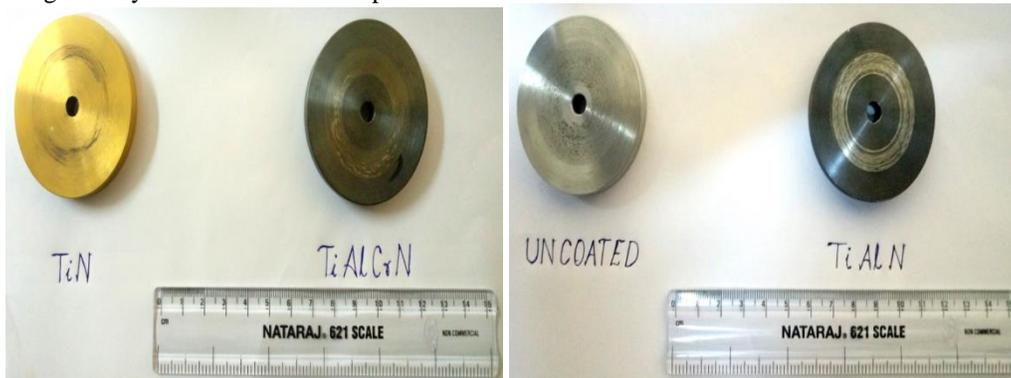
Fig. 2: Shows of Coated and Uncoated materials
