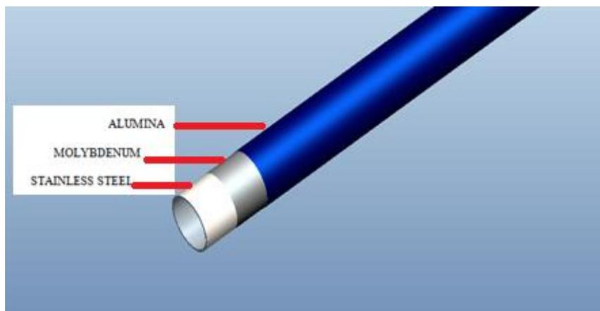
Fig. 3: Mo/Al<sub>2</sub>O<sub>3</sub> coating on absorber tube
