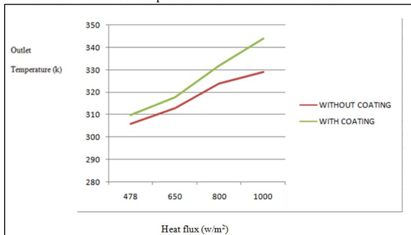
Fig. 9: Outlet temperature vs Heat flux
