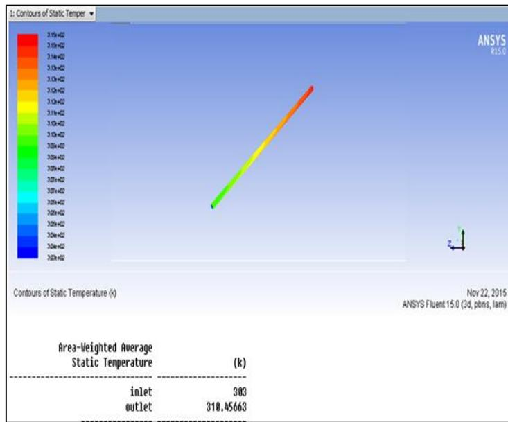
Fig. 7: Temperature distribution with coating
