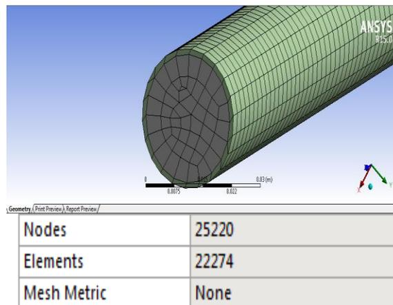
Fig. 4: Meshing of absorber tube without coating
