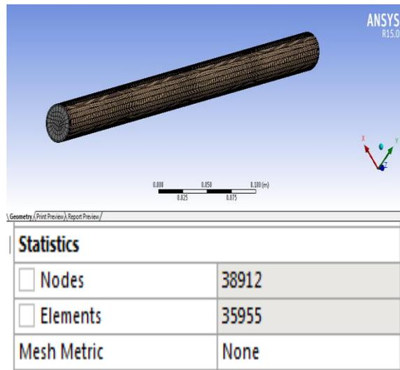
Fig 5: Meshing of absorber tube with coating
