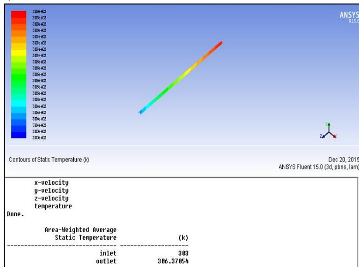
Fig. 6: Temperature distribution without coating
