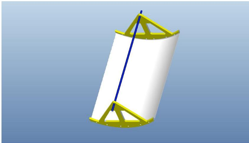
Fig. 2: 3D view of parabolic trough
