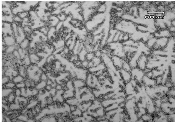
Fig. 5: Optical photomicrographs of AA 2219 + TiCp 7%
