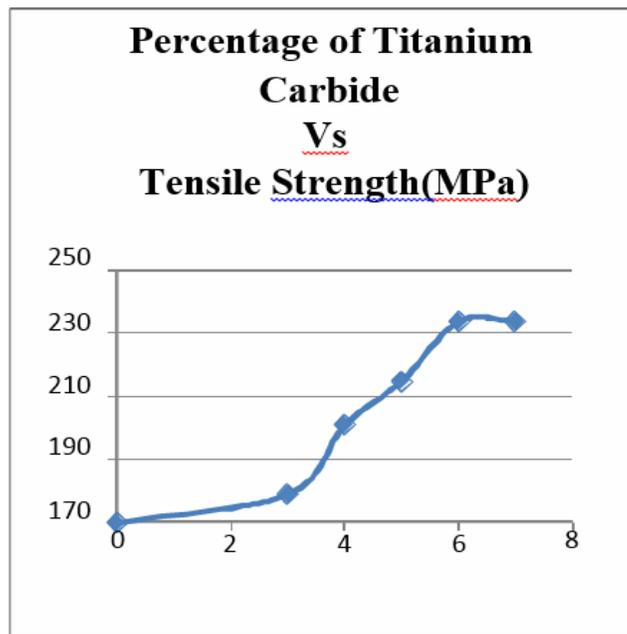
Fig. 2: Percentage of TiC<sub>p</sub> on Ultimate Tensile Strength.
