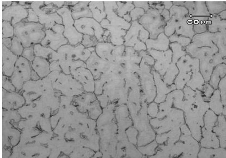
Fig. 4: Optical photomicrographs of AA 2219+ TiCp 3%
