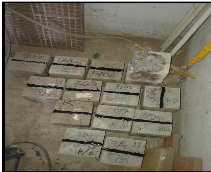
Fig. 3: Crack filled by bacteria
