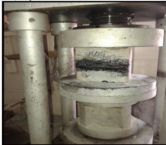
Fig. 4: Compression test on concrete cube after filling crack with bacteria + rise husk ash
