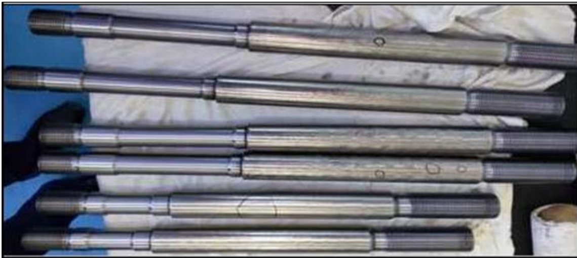
Fig. 2: Piston Rod Defect Photograph (Porosity)
