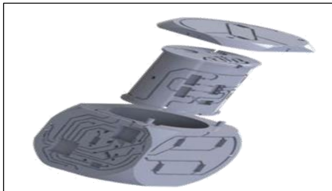
Fig. 2: 3D Printed Electronic Device without Components
