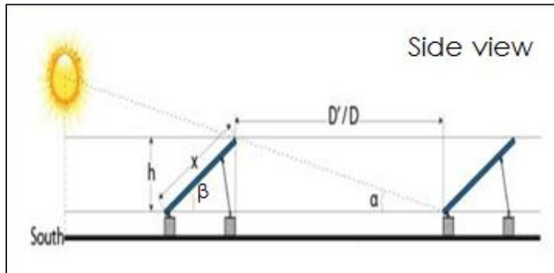
Fig. 3: Inter array spacing calculation-Side view
