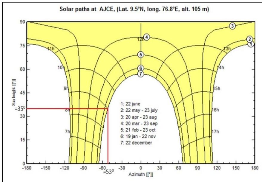
Fig. 6: Sun path chart generated using PV Syst software
