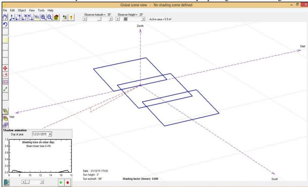
Fig. 7: Shadow calculation using PV Syst software
