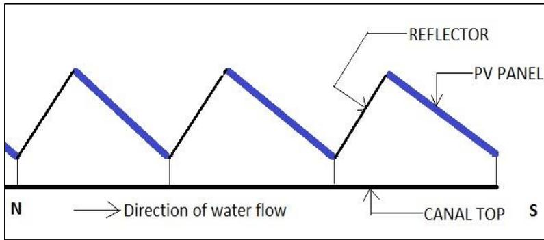
Fig. 2: Canal top project with reflector in the inter array spacing
