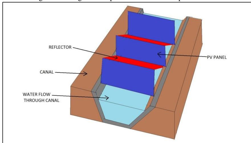
Fig. 5: Canal top project with reflector in the inter array spacing
