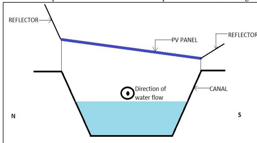
Fig. 1: Canal top project with reflector on sides
