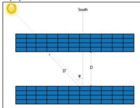
Fig. 4: Inter array spacing calculation-Top view
